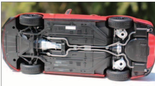
*The chassis is well detailed and has a fully articulated four-wheel independent suspension.*
