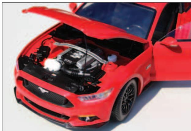
*The Mustang's engine compartment includes the shock tower brace used to stiffen the suspension.*
