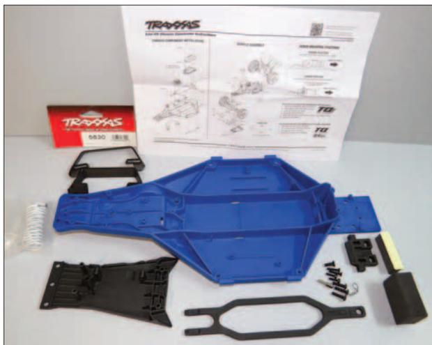
*The Traxxas kit contains everything needed to lower the battery and motor in a Slash one inch.*
