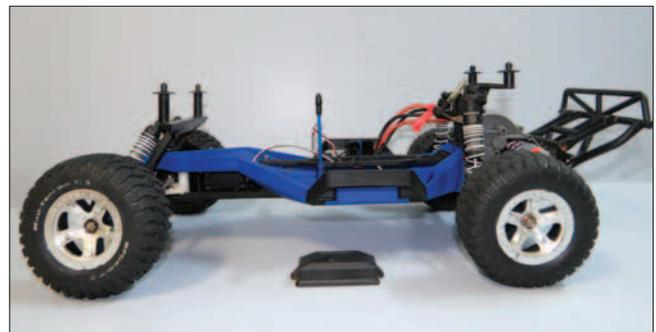
*Ground clearance remains the same, but lowering the battery and motor definitely improves handling.*
