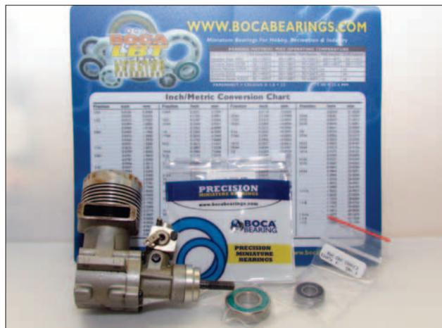
castor or model engine oil. When working on the internal parts of any engine, avoid metal tools. The tiniest burr or scratch can be the end of a successful repair. For the internal work you will need some hardwood or synthetic dowels, and a small plastic head hammer. Lastly you will need a pair of oven mitts to protect your hands during the bearing removal and replacement process.
