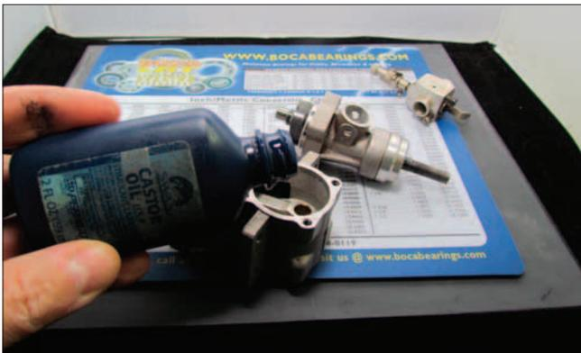
*A light application of oil during reassembly will protect the engine during the initial start up.*
