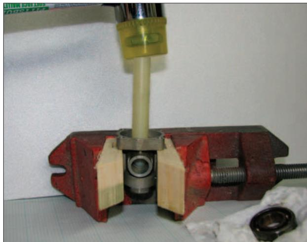
*For this repair, the front bearing was gently tapped out of the crankcase using a Delran rod.*
