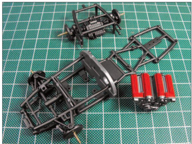
*Frame and suspension parts were painted steel, a dark color that provides contrast to the many detail parts that are added as assembly of the model progresses.*
