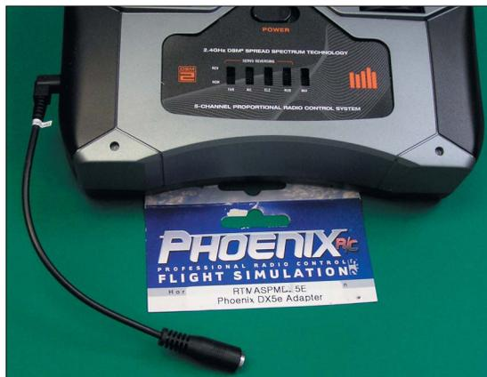
*The Phoenix comes with a cable to adapt the DX5e to the simulator. Cables for other brands are also available.*
