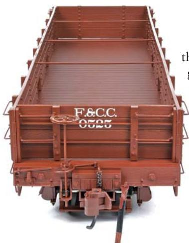
View from the B end shows the cross rods that support the sides and keep them from bowing outward under load. You can also see the wealth of detail in the brake and draft gear. This particular car has already been converted to Kadee couplers.
