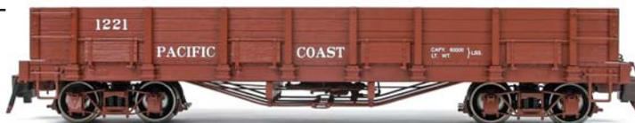
HM's two samples show the Florence & Cripple Creek No. 0525 from Central Colorado and the Pacific Coast No. 1221 from the South Pacific Coastal region. Both are truss rod type side dump-style gondolas, typically built from 1890 to 1910.
