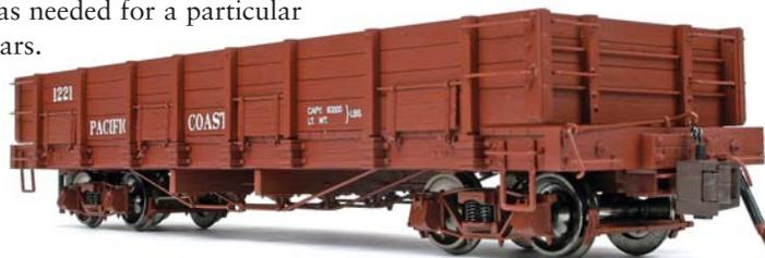
This 3-quarter A-end view shows the authentic step straps and how the narrow gauge trucks are tucked underneath. This is a pre-coupler conversion shot with the cut bar connected to the lift pin on the Bachmann coupler. The air hose is a wonderful bit of business.
