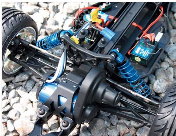
*Rugged suspension, oil-filled coil-over shocks and a wheelie bar all hint that the Xcelorin Brushless motor really rips.*
