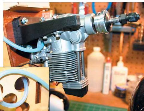
O.S. FS-120 Surpass III with Pump fits neatly inside the Hawk's huge fiberglass cowl. Note use of Great Planes Easy Fueler Fuel Filler Valve (GPMQ4160) and Sullivan Products Head Lock Remote (MO21) for cowl-on service access.
