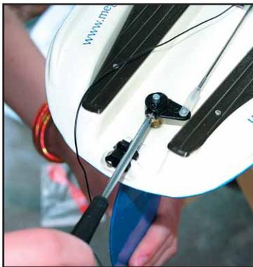
Devin Troy tightens the set screw to secure the rudder's tiller arm.
