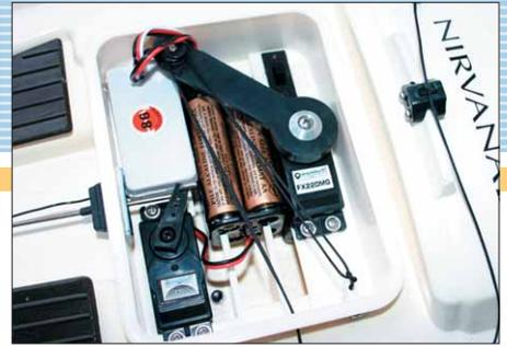
Nirvana II's removable ballast keel inserts from beneath the hull and locks with a twist tab. New sail servos have increased torque.
