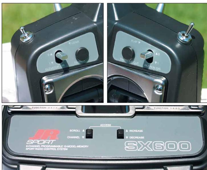
*JR SPORT RC systems come in four-channel and six-channel versions, the latter having more programming options, dual rates and exponential on the aileron and elevator channels. Programming these radios is intuitive, with simple and logical commands that anyone can learn quickly.*
