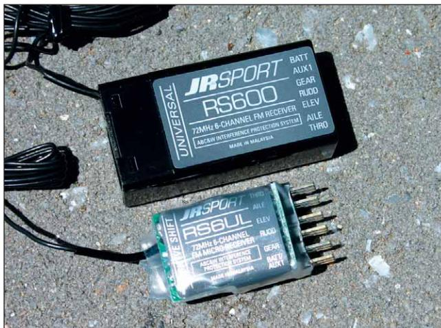
Two FM receivers serve JR SPORT. The RS6UL Micro is available in Positive and Negative shift versions. The RS600 is a Universal Receiver, shifting between Positive and Negative with a jumper.
