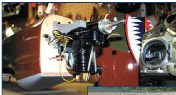
*Saito FA-100 GK four-stroke fits perfectly in the Warhawk's painted fiberglass cowl. Cavernous fuselage holds receiver, battery and throttle servo with room to spare. Rudder and elevator servos at rear of fuselage.*
