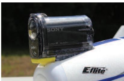
A Sony camera was mounted to the recess located on top of the fuselage, and although a clean installation, the location of the camera's controls made operation difficult. Decided upon was a Hero-3 mounted to a simple snap connector that allows the camera to be taken on and off as desired.
