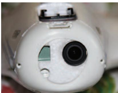
One of the nose inserts is for a Go-Pro style of action camera and it includes openings for access to the camera's various function controls.
