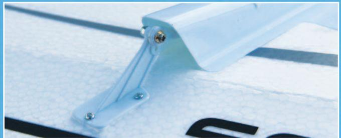
Potential glue joint failure has been eliminated by screwing the control horns to the elevon surfaces and using through bolts and lock nuts on the horn to servo connections.
