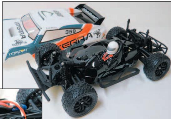
*Top: What appears to be a driver's bust and interior is actually a cover to protect the radio equipment. Left: the chassis components are waterproof, and the layout is neat and orderly.*
