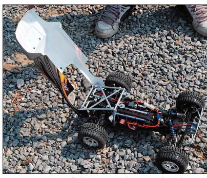
service easy. A large, coil-over shock is at each of the four corners, and a very cool lighting system gives good visibility and great visual effects for night runs.
