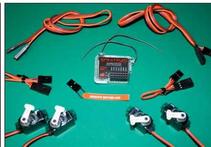
servos, and E-flite's Foam Safe CA for all other foamie construction. The rudder and elevator servos mount in the rear of the fuselage, and use 18-inch extensions to reach the receiver. All these are easiest to install before the wing. Installing the horizontal stabilizer completes the entire airframe assembly.
