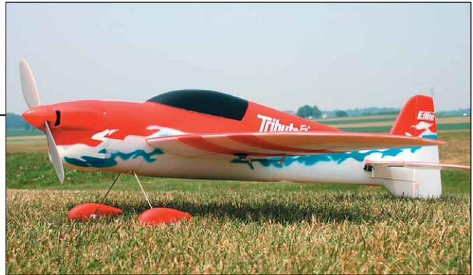
High Power Outrunner Setup, which recommends the Park 450 Brushless Outrunner, E-flite's 20A ESC and a Thunder Power 3S 1320mAh LiPo pack. I also chose my Spektrum (love those 2.4GHz RC systems) DX7 with an AR6000 receiver and four E-flite S-75 Sub-Micro Servos.
