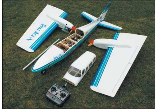
*Setup is quick. Hex socket screws hold the canopy, and four nylon bolts secure the wing panels, which slide over the joiner.*
