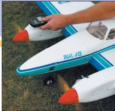
*Engine accessibility is excellent without removing the fiberglass nacelles. Needles, glow plug and fuel lines can all be easily reached for startup or service. Tach is a good idea, and a short glow driver is needed for the port engine.*
