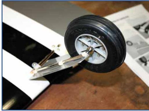
*Hangar 9 Mustang PTS flap linkage is installed in the down position for primary training, and can later be raised or servo operated for intermediate flight. Flap servo cutout is provided in wing center section. Speed brakes come attached to landing gear legs for basic training, and these parts are also removable for intermediate flight.*
