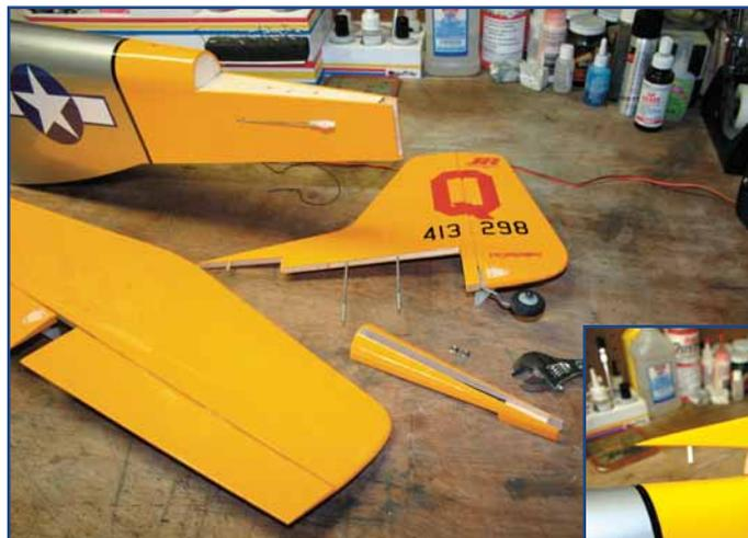
*Horizontal stabilizer and vertical fin fasten to rear of fuselage in typical ARF/RTF fashion. Tip of dorsal fin uses dowel pin to maintain alignment.*
