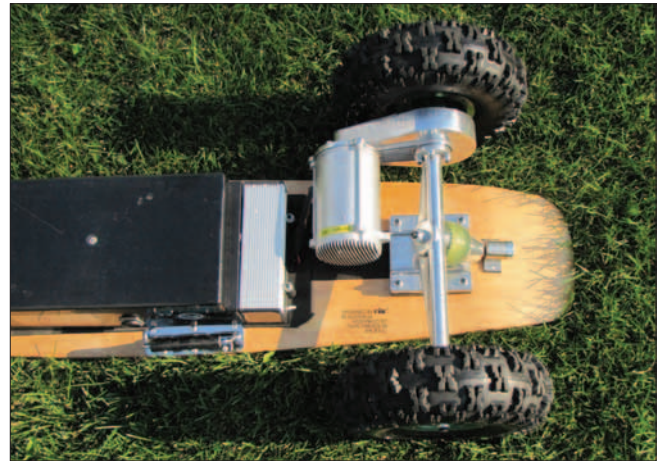
The trucks are manufactured from an aluminum alloy and like the entire product are well engineered.
