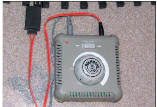
*The speed controller is a standard Bachmann analog unit featuring a large dial, and ease of operation.*
