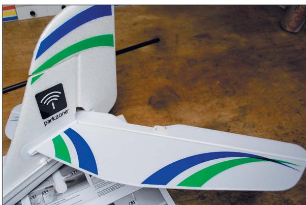
Stabilizer slips through slot in fuselage, and is secured with four strips of tape. Connect the clevis to complete the tail.
