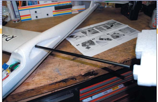
*Wing panels slide over carbon joiner rod, and press-fit into a central fuselage cavity. The assembled wing is very strong.*
