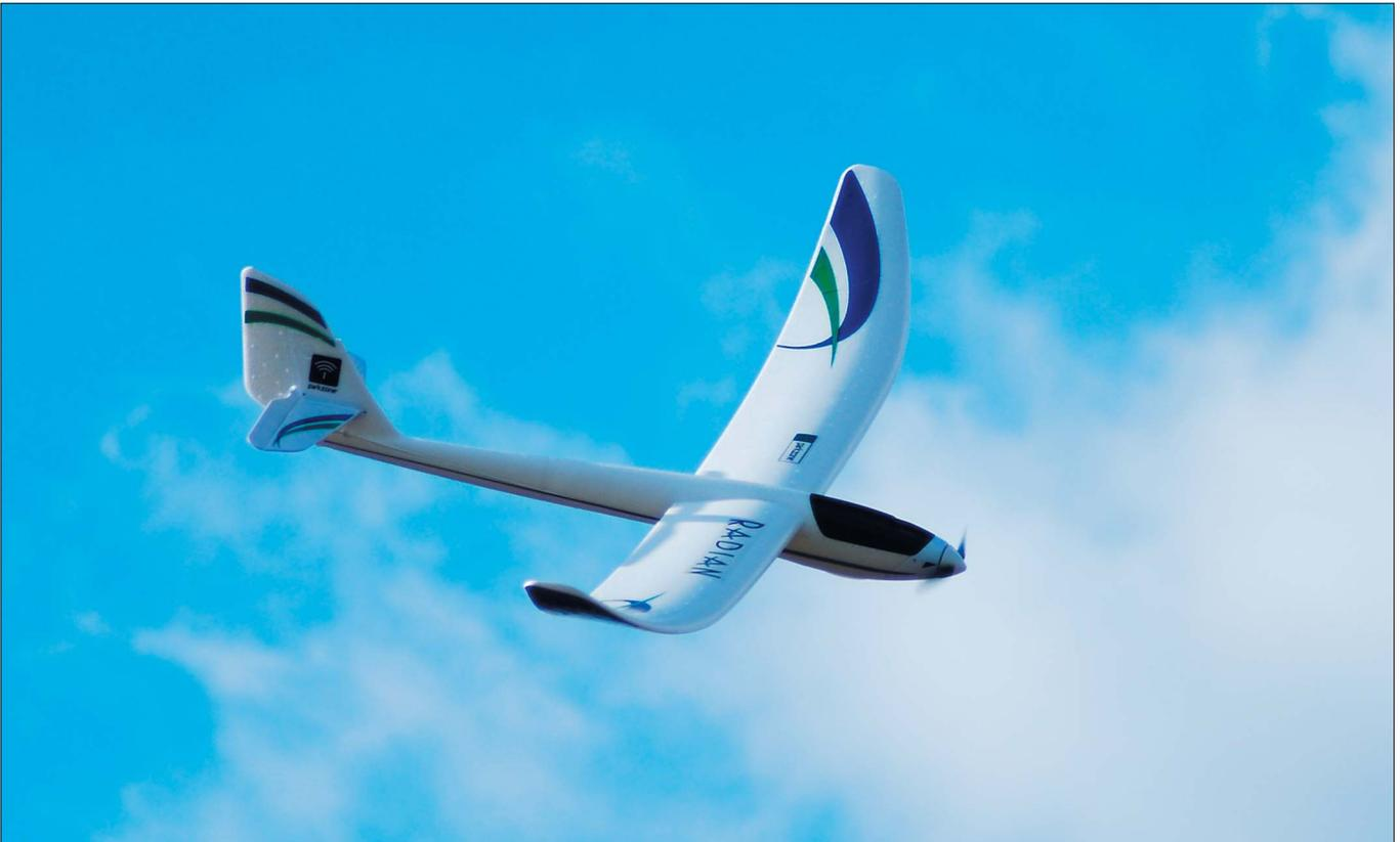
*It's hard to beat the sight of a sailplane in lift, and the motor glider features completely negates the need for a hi-start or winch launch.*
