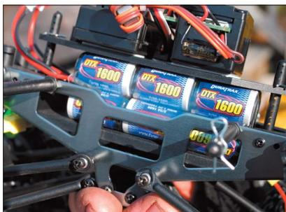
Two DuraTrax 7.2-volt 1600mAh motor batteries and eight AA alkaline cells for the transmitter are the only extras needed. Everything else is included in the RTR.
