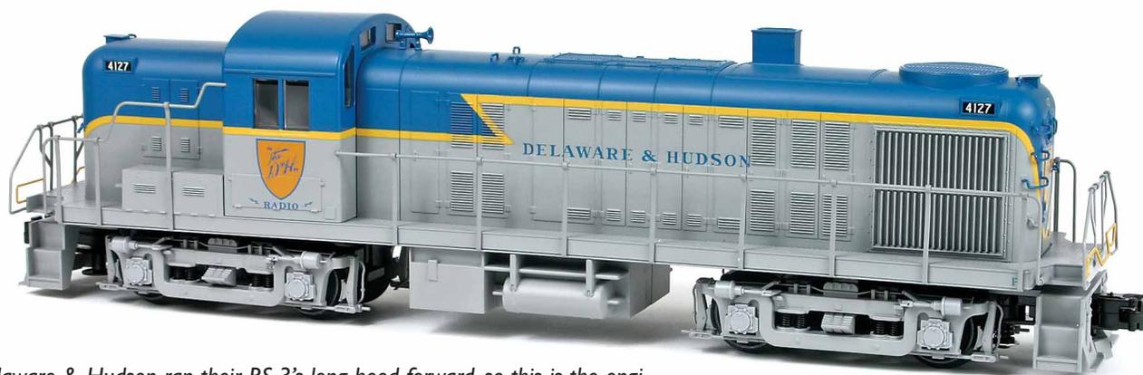
*Delaware & Hudson ran their RS-3's long hood forward, so this is the engineer's side of the locomotive. For what is supposed to be a low-priced, entry-level piece, this is a feature-rich and good-running model.*
