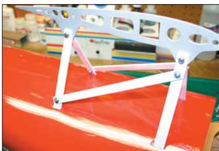
Sturdy aluminum cabane strut assembly is fastened to aligning structure below the deck with socket head cap screws and Nylock nuts.
