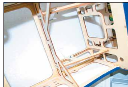
Sturdy aluminum cabane strut assembly is fastened to aligning structure below the deck with socket head cap screws and Nylock nuts.
