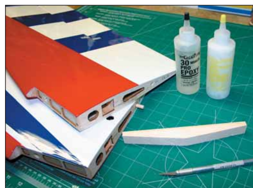
Factory-assembled and MonoKote covered wing panels are joined with 30-Minute Pro Epoxy by Great Planes.
