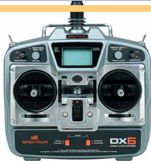
The Spektrum DX6 is a six-channel computer system, exclusively designed for park flyer airplanes and micro/mini helicopters. Although it carries a “park flyer” nametag, one shouldn’t be duped into thinking that this is a beginner’s radio system. The Spektrum DX6 is a full-blown computer radio with a 10-model memory and plenty of programming, but those are a just a few short notes in the Spektrum’s song. Just wait until you hear the rest of the tune.
