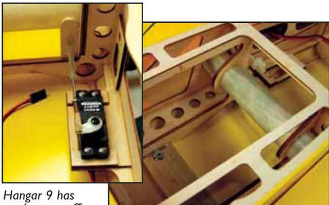
*Hangar 9 has made every effort to keep this model as light as possible. Interlocking, laser-cut construction assures maximum strength and minimal weight.*
