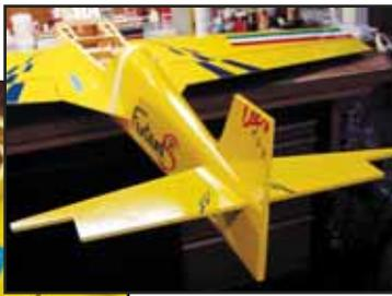
*Trailing edge root fillets are secured to the wing panels, then the horizontal stabilizer and the vertical fin are*
