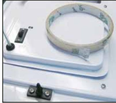
*RC compartment is sealed with supplied clear waterproof tape. Stern post engages removable deck, retained by a hairpin clip.*
