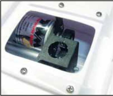
MegaVolt nickel-metal hydride pack from Megatech International, along with their simple MegaPeak AC/DC fast charger. This setup allows for run times of 8 to 9 minutes at full speed.
