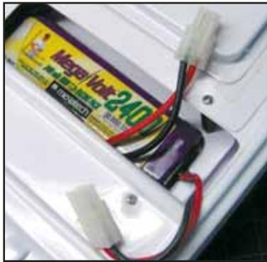
*Battery bay holds 6-cell motor pack. Tamiya-style connector.*
