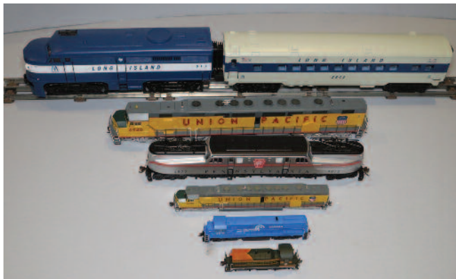
Consideration also needs to be given to the type of locomotives and rolling stock the budding enthusiast is interested in. As an example even though the Union Pacific EMD DDA40X and the GG1 are shown in HO (half-O for those not in the know) locomotives for this size will still require a minimum of a 36-inch radius turn to operate correctly, whereas an N-scale switcher style of engine will easily operate on a layout as compact as two feet in total width.
