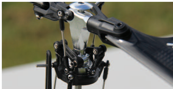
While the main rotor head is machined aluminum, the swash plate is a robust composite structure. All of the control links feature metal balls for precision control and under normal use the stock swash will last the owner a considerable length of time before needing replacement.
