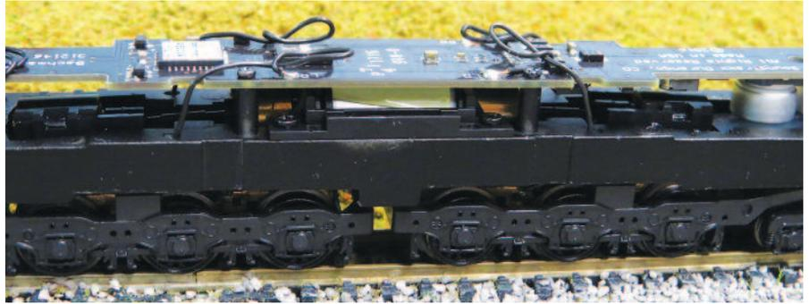
The heart of the locomotive is a circuit board that is mounted on top of the drivetrain and runs the full length of the locomotive. The board not only contains the DCC circuits for superb scale-like operation, but also the SoundTraxx sound system and even a tiny speaker.
