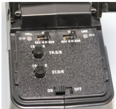
With either version the included transmitter is a full-size pistol grip unit that features all of the basics such as throttle forward and reverse along with steering forward and reverse and centering trim for both throttle and steering.
