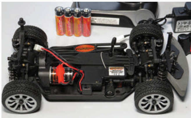
The chassis is low-slung which makes for a road hugging center of gravity and is equipped with some sticky tires which results in rather amazing road holding ability. Shown is the brushed version, and other than the motor the only real difference between the vehicles is the two-in-one receiver/ESC incorporated in the lesser expensive brushed version.
