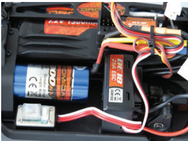
The brushless version accelerates faster and is noticeably quicker than the brushed version. It also utilizes a separate receiver and 25 amp ESC. With either version the electronics are listed as waterproof, but that doesn't mean the cars are to be used as submarines.
