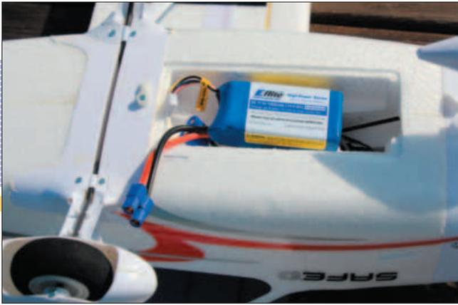
*There is plenty of extra room in the molded battery compartment, making replacement and/or charging an easy process.*
