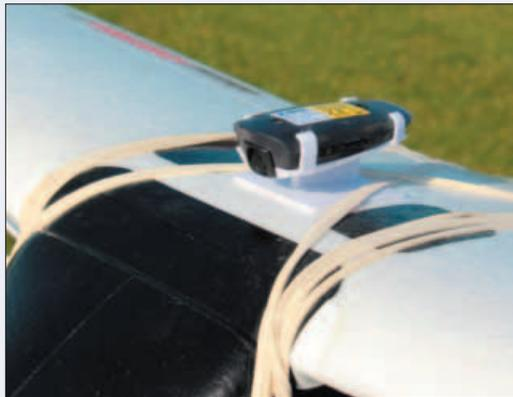
light weight (15 grams), hi-definition camera that's even aerodynamic in its shape, EFC-721 HD Camera (EFLA801).
