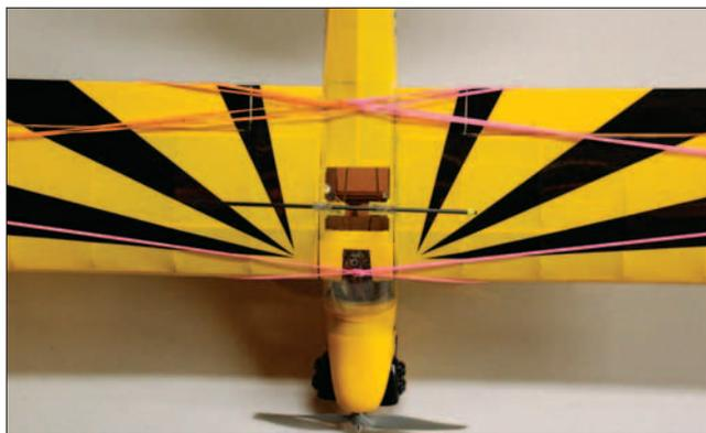
*The manual dictates adhering the wings to the cabin structure, but they could be made removable if space is at a premium.*
