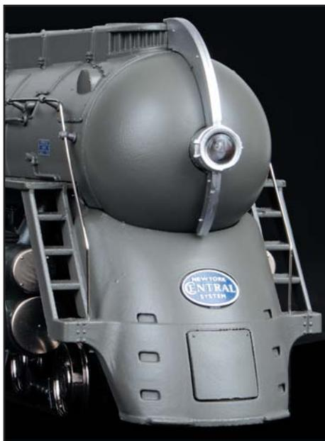
*This is the face of the Art Deco movement, complete with the cutlass down the nose, splitting the wind, and stirring excitement in watchers. Under the pilot panel is the swing-out dummy coupler. You can also install a magnetic knuckle coupler there, if you wish.*
