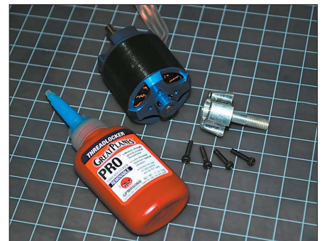
Propeller adapter fastens to the motor case with four socket head cap screws.
