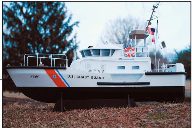
using penny rolls wrapped in clear plastic; a roll of pennies weighs 5 ounces. My dad and I discovered that the ballasting process can be one of trial and error. I began driving the Motor Lifeboat only to realize that the balance was off. We brought it back to shore, did some adjusting, and sent it back to “sea” with better balance.
