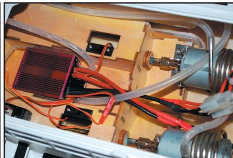
Pro Boat 75MHz RC system has trims and reversing. Twin water-cooled motors and ESC provide plenty of go. Note switches for RC and nav lights.
