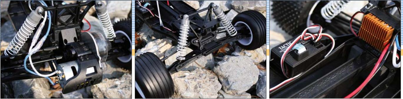
*DuraTrax Evader EXT RTR carries a 540-size Photon Speed 2 brushed motor for clean and economical running. Oil-filled, coil-over shocks keep the suspension working at its best. High mounted ESC with large heat sink keeps unit consistent under extreme conditions.*
