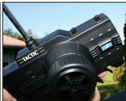
*TACTIC brand is a Great Planes exclusive. The pistol-grip transmitter features throttle and steering trims, and the rate knob allows precise adjustments for steering on the fly. The receiver, steering servo and ESC are factory installed.*
