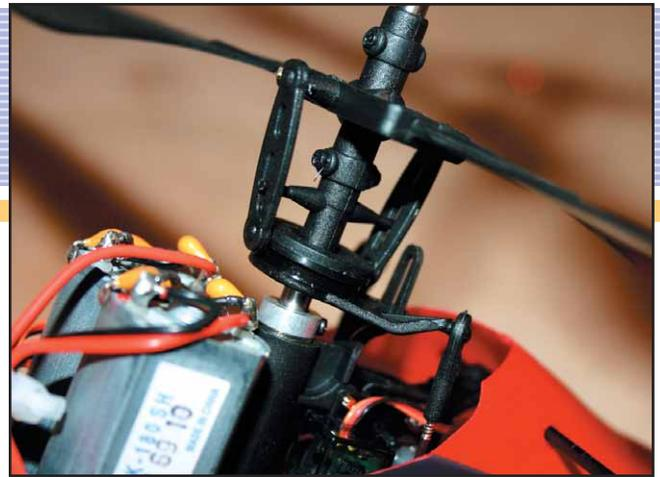
*The heart of the Blade CX2's success is its simple head and dual coaxial rotor system. The machine practically flies itself.*
