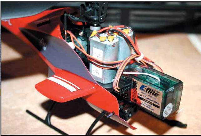
*4-in-1 Control Unit has improved gyro for greater tail control and less drift. S-60 Super Sub Micro Servos are light and fast.*
