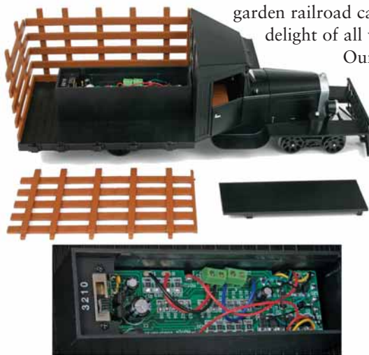
Power board inside bed box, covered by snap lid. Power switch is on left while the rest of the board is laid out for easy access.
