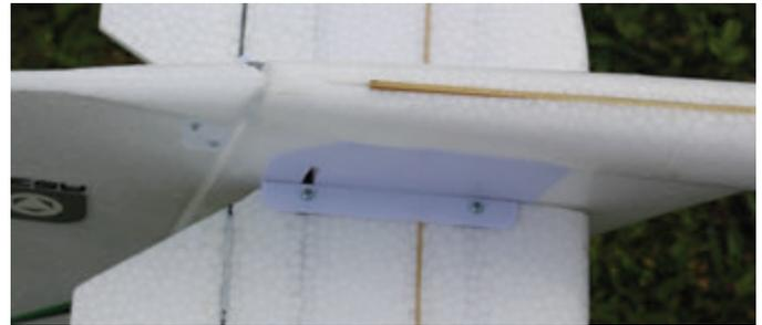
The horizontal tail utilizes stabilator (stabilizer and elevator combined as one surface) control. The halves are secured to two carbon fiber spars by using same diameter, but different length machine screws. Instruction manuals are printed for a reason and to avoid disappointment the end user absolutely must read and follow the manual.
