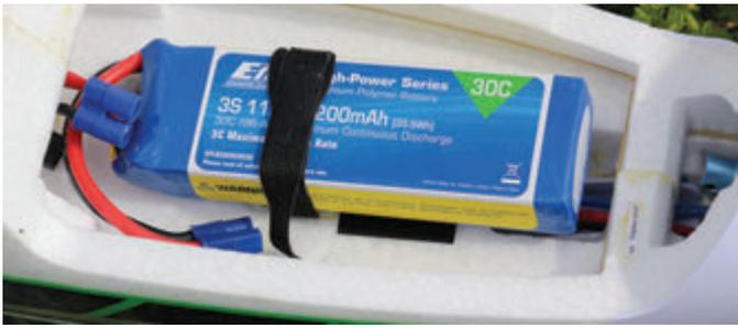
Located under the removable canopy is a huge battery compartment, which allows for plenty of fore/aft placement of the recommended 3S 3200mAh flight battery to help with any balance issues.
