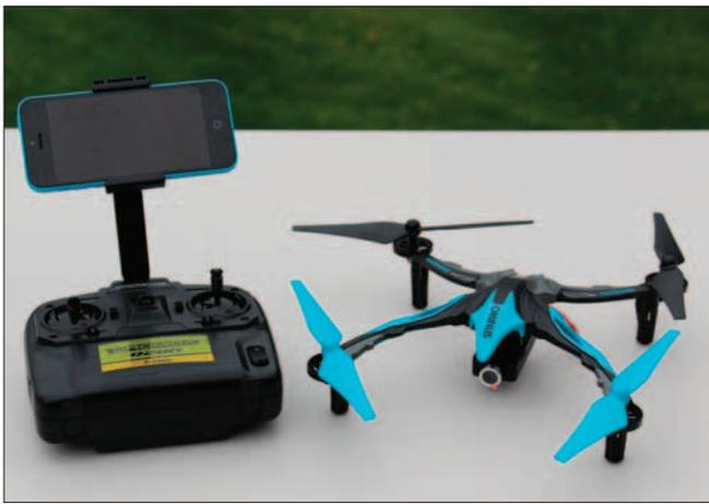
*The Ominus FPV includes a bracket for the transmitter so a smart phone can be mounted as a monitor.*
