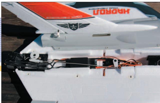
*The mount for the vertical stabilizer also doubles as a cover for the speed control along with the rudder and thrust servos.*
