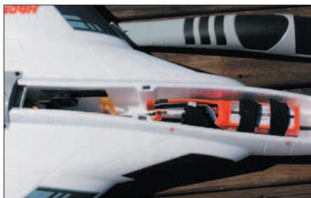
*Above: Removing the canopy hatch reveals a large compartment that will accept a variety of 3S and 4S battery packs. Right: The elevon servos are glued in pockets that are molded into the wing and use short pushrods for slop-free control movement.*
