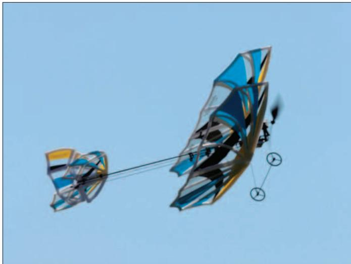
*Two complete airframes are contained in one box, allowing the purchaser to select between a monoplane or the biplane (shown).*
