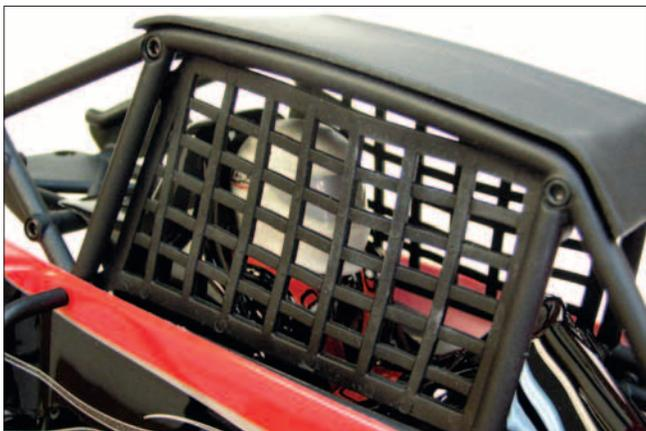
There are a number of scale details present, like the simulated webbing designed to keep the driver's head inside the full-scale buggy during a roll-over collision.
