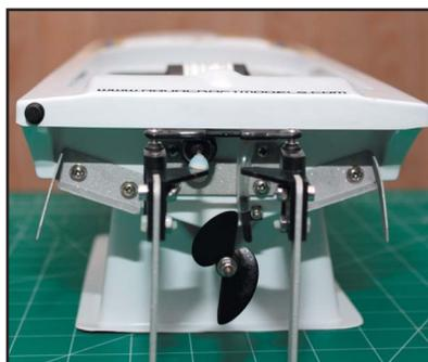
Twin rudders not only look good but provide for precise steering. Items such as trim plates, turn fins and the rudders can all be polished if the customer is interested in racing.
