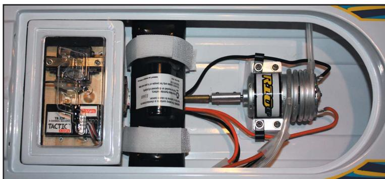
The interior of the boat is well laid out with the receiver, steering servo and ESC all contained in a separate waterproof radio box. Shown is an 8.4 volt hump pack battery, which is held in place by hook-and-loop straps.
