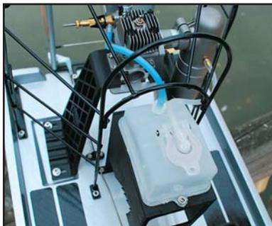
Next, use a #1 Phillips screwdriver to remove the two Phillips head screws from the top of the radio box. Take off the seat assembly and the radio box cover, then install the other four AA batteries in the battery holder. Slip the battery box back into the radio box, replace the cover and
