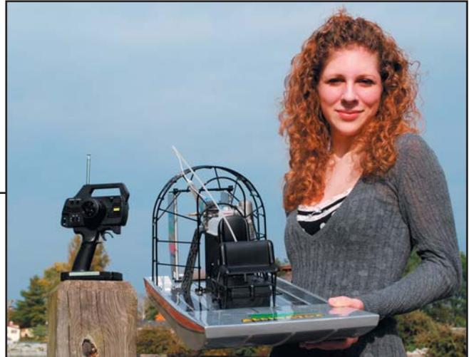
The first step is to screw the antenna into the transmitter, then remove the battery door from the bottom of the handle. Then, being sensitive to polarity, insert eight of the 12 AA batteries and reinstall the door. Turn the transmitter to "on" and the LED should glow green. If it blinks red, the batteries need to be reinstalled or replaced.
