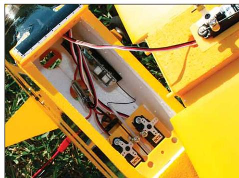
Tactic RC system with three micro servos and an auto cut-off electronic speed control comes factory installed.
