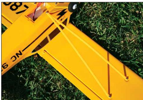
Each wing strut attaches with three Phillips-head screws, and FlyZone even includes the correct size screwdriver.
