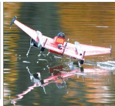
*HydroFly builds up speed on water and begins to plane, then pilot hits and holds Takeoff Activator button to rise from the surface. Once airborne, one of the four available motor speed steps is selected to maintain straight and level flight.*
