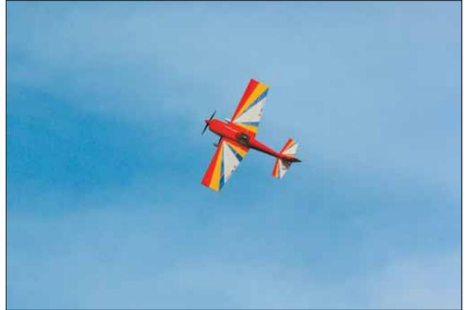
*Maximum rudder throw is mandatory for knife-edge flight.* stability, but still leap aggressively at every command when the sticks are thrown a little farther. The rudder should be set for extreme deflection if knife edge flight is to be performed with any authority. Rudder wag should almost contact the elevator panels at full deflection.
