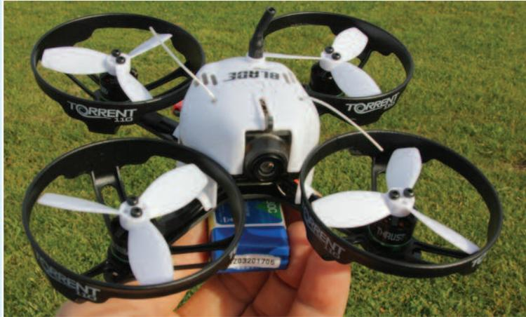
It may be small, but don't be fooled by the size. The Blade Torrent 110 FPV is well mannered and a delight to fly on a 2S flight battery, but step up to a 3S flight pack and wow, the machine is nothing short of ballistic.
