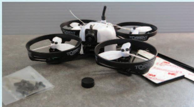
The FPV camera is mounted to the top of the chassis and is covered by a lightweight molded body. Actually there is nothing that is part of the platform that is not needed for flight. This includes landing gear, as the machine simply rests on the flight battery when preparing to takeoff or when landing.
