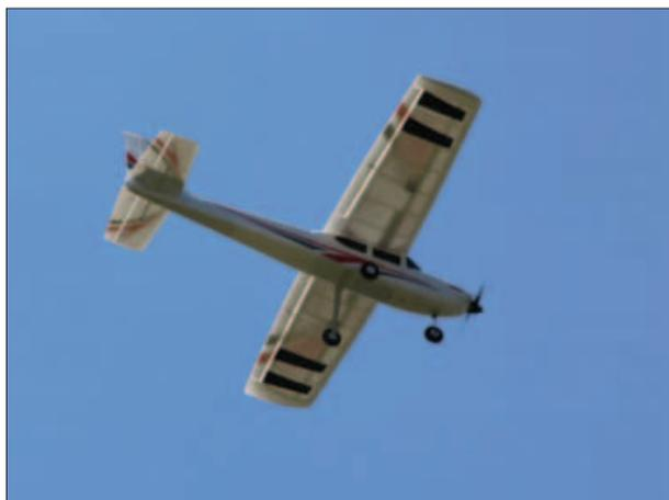
*A colorful trim scheme, to help in visual orientation, is as important to the new pilot as the electronic stabilization.*
