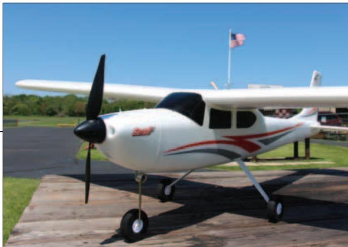
Sensei is a nice size for a trainer. It's not too large of a model to conveniently transport, and it's not so small that the student is constantly plagued with making turns to keep the model orientated. Manufactured from the company's AeroCell, the Sensei is by no means the largest molded foam aircraft, but it is relatively large for a foam product, and as stated, it's a nice size for a trainer.
