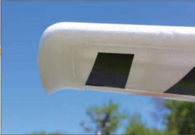
*Beyond the WISE stabilization system, the Sensei incorporates additional aerodynamic aides, such as the Horner wingtips.*
